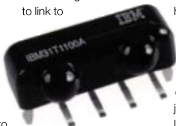
An IBM 31T 1100A infra-red transceiver chip
